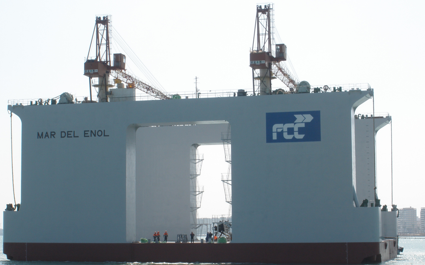
The Mar del Enol floating dry-dock was used for the first time to manufacture the caissons for the Port of Açu (Brazil).
