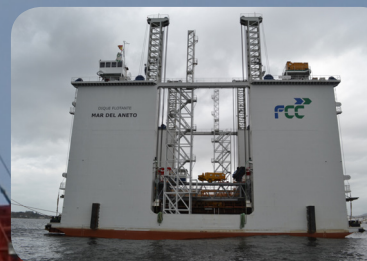
Mar de Aneto, the floating dry-dock designed for building breakwaters, docks, and jetties is 46.8 metres long and 32 metres wide.
